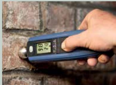
**APPLICATION** It is of importance **how the unit is held** while measuring: The **BL Compact B** unit should be held at the rear part of the unit and applied to the material to be measured in a 90° angle.
